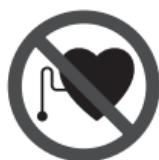
**Keep the measuring tool away from cardiac pacemakers.** The magnet plate 5 generates a field that can impair the function of cardiac pacemakers.
